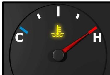
There are two primary types of coolants available on the market today. The first is traditional, green-colored antifreeze, which can be used in any car. The second is a newer, long-life coolant, which comes in a variety of colors. It should only be used in recent-model cars because it may damage some of the engine gaskets in older cars. If you're not sure whether your car uses the new or old-style antifreeze, check with your manufacturer.
